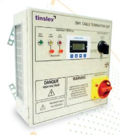
It offers a simple method of selecting an open or short circuit condition and a safe means of discharging the cable. The unit is designed to enable the Test Engineer to safely and simply connect other Tinsley test instruments to the system for fault location and electroding.
