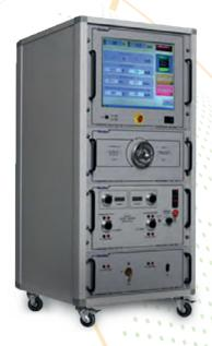
The more common test procedures which are associated with the location of types of cable fault such as 'open circuits' and 'shunt faults' are preprogrammed into the instrument. This allows the procedure to be carried out automatically therefore eliminating operator errors and reducing the uncertainty of the predicted fault position.
